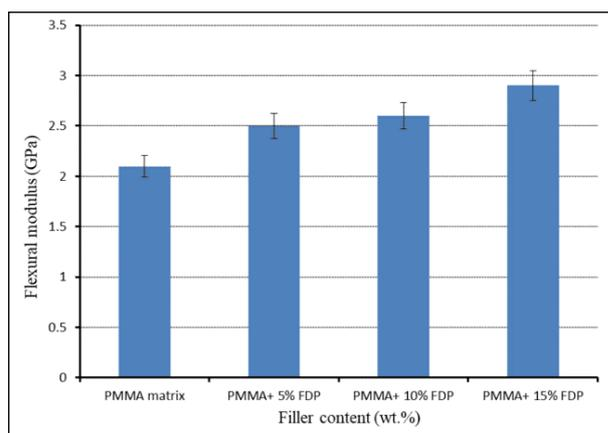
Fig 9. Flexural modulus of PMMA and PMMA/FDP.
