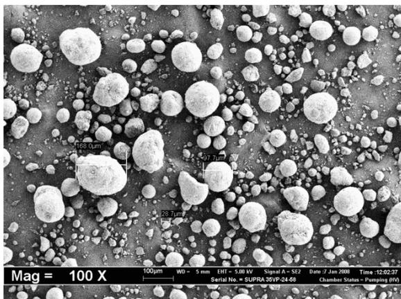
Fig 5. Micrograph for Silica.
