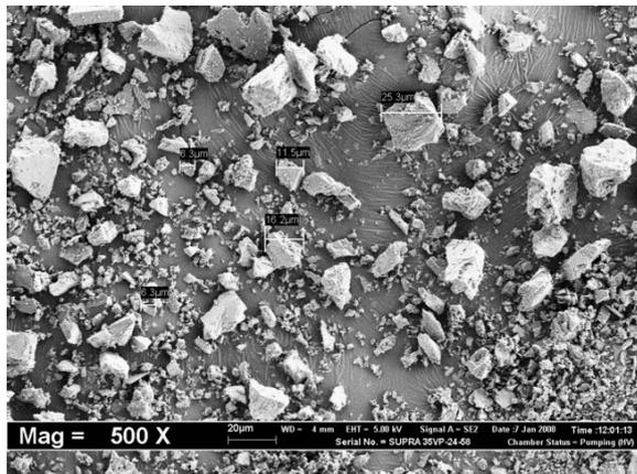
Fig 4. Micrograph for Na-feldspar.
