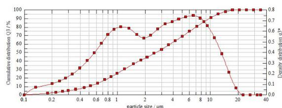
**Fig 6.** Particle size distribution of FDP particles.
