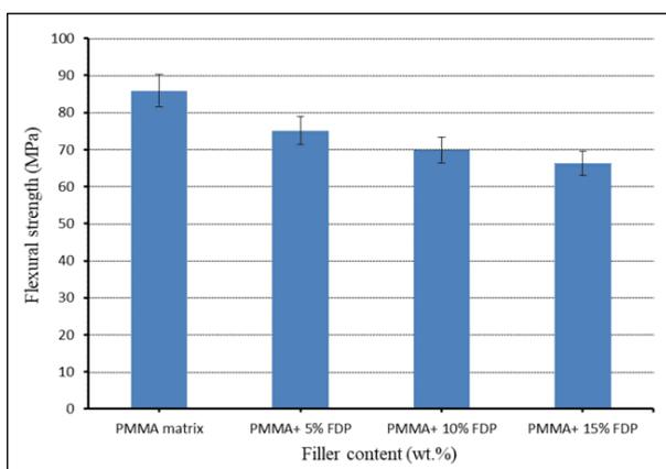
Fig 10. Flexural strength of PMMA and PMMA/FDP.
