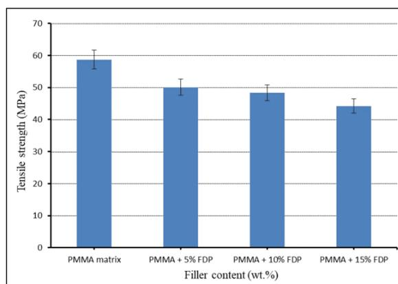
**Fig 8.** Tensile strength of PMMA and PMMA/FDP.
