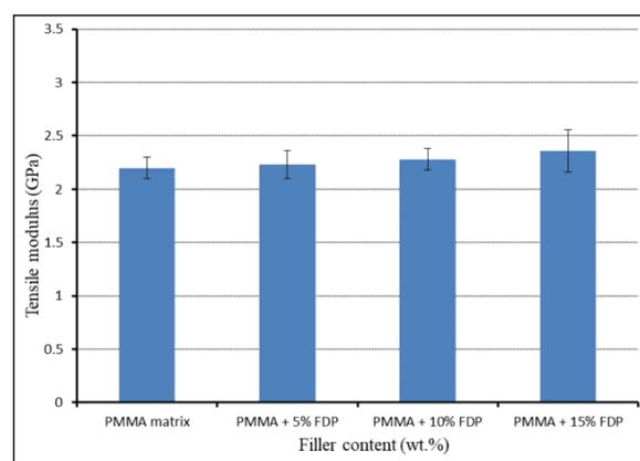
**Fig 7.** Tensile modulus of PMMA and PMMA/FDP.
